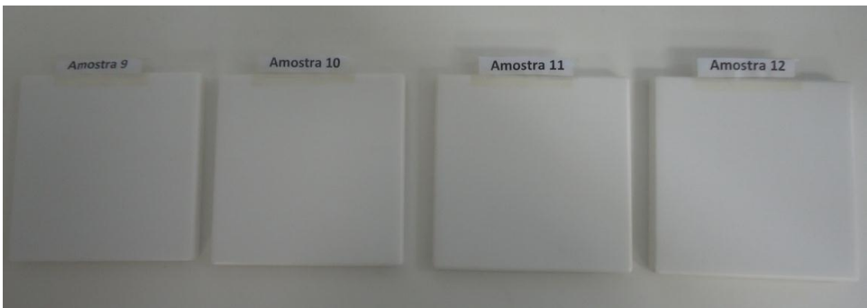
Figure 6: Corian® steel plates before starting the test. Sample 9: removal of the product after 10 minutes; Sample 10: removal of the product after 20 minutes; Sample 11: removal of the product after 30 minutes; Sample 12: without removal of the product.
