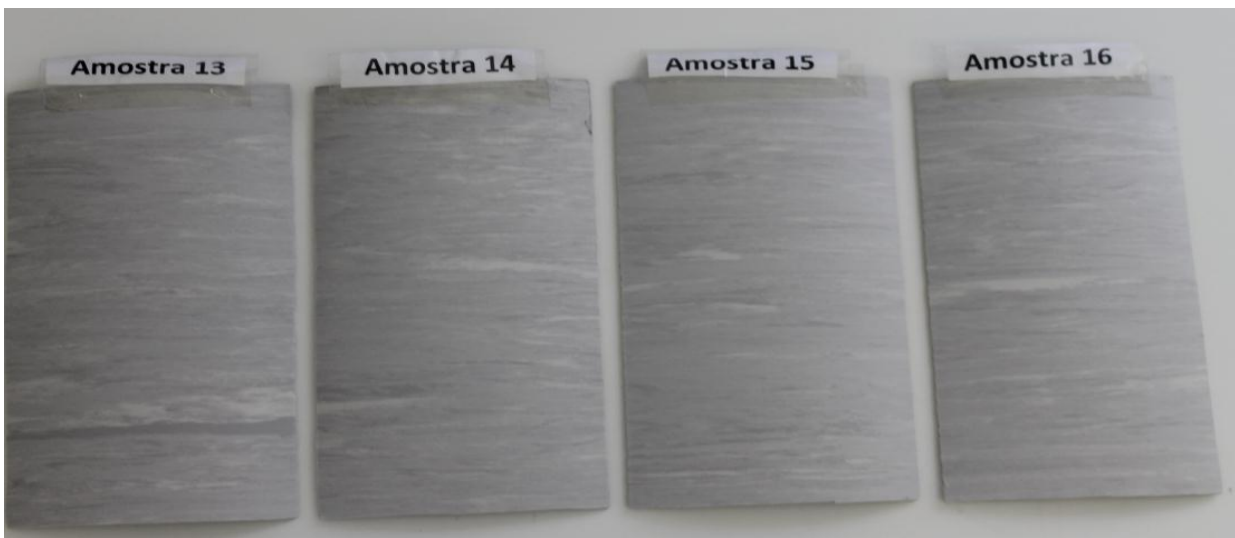
Figure 9: Vinyl floor tiles after 12 weeks of testing. Sample 13: removal of the product after 10 minutes; Sample 14: removal of the product after 20 minutes; Sample 15: removal of the product after 30 minutes; Sample 16: without removal of the product.
