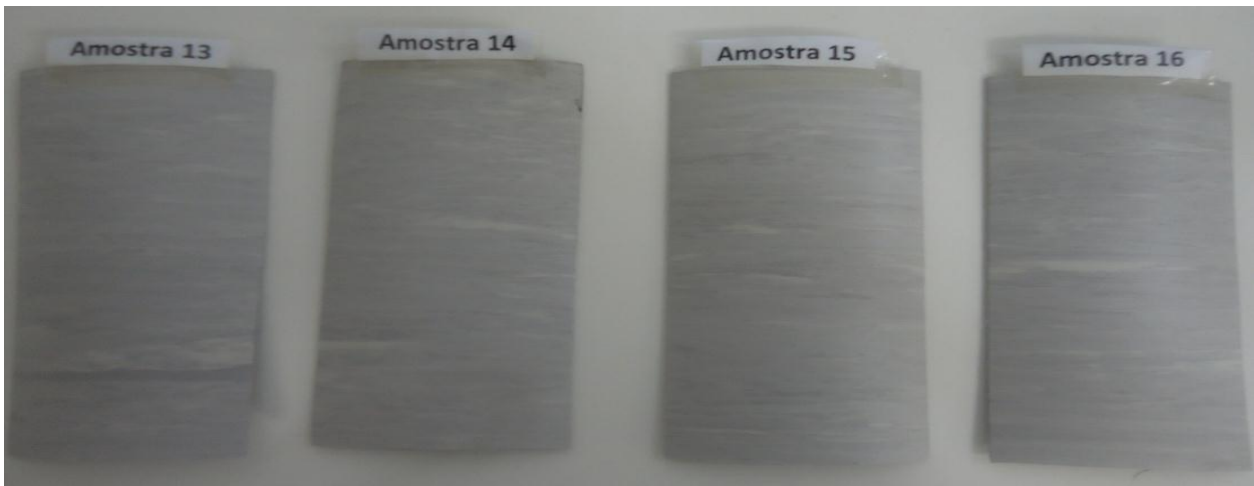
Figure 8: Vinyl floor tiles before the test starts. Sample 13: removal of the product after 10 minutes; Sample 14: removal of the product after 20 minutes; Sample 15: removal of the product after 30 minutes; Sample 16: without product removal
